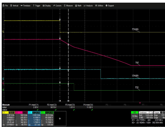
Figure 5: AIF04ZPFC-01L Turn-off Characteristic via PF ENABLE Vin = 115Vac Load: lo = 0A Co = 470uF Ch 1: PF ENABLE Ch 2: Vo Ch 3: LD ENABLE Ch 4: PFW
