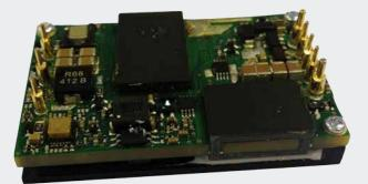
Advanced Energy's Artesyn AVQ100-36S3V3 is a single output DC/DC converter with standard quarterbrick outline and pin configuration. It delivers up to 25A output current with 3.3V output voltage.
