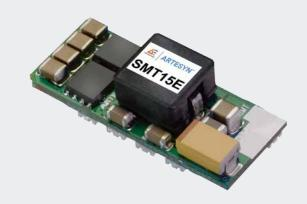
Advanced Energy's Artesyn SMT15E series of non-isolated DC-DC converters comprises two fixed output models offering voltages of 2.5 V or 3.3 V, and one wide output trim model that can adjusted over the range 0.8 to 3.63 Vdc. All three models can deliver up to 15 amps output current. The 3.3 V fixed output model accepts a 4.5 to 5.5 Vdc input, while the other two models accept a 3 to 5.5 Vdc input.
