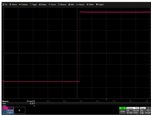
Figure 11: AIF42BAC-01N Output Voltage Startup Characteristic Vin = 230Vac Load: I o = 42A Ch 2: V O
