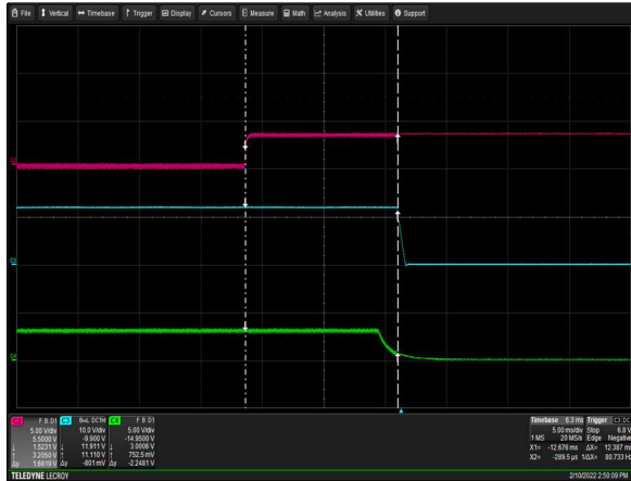
Figure 7: AIF42BAC-01N Turn Off Characteristic via PS_ON Vin = 230Vac Load: I o = 42A I SB = 0.25A Ch 2: PS_ON Ch 3: V O Ch 4: PSU-Good
