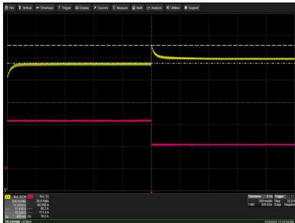
Figure 9: AIF42BAC-01N Transient Response - V O Deviation 100% to 50% load change 1A/μs slew rate Vin = 230Vac Ch 1: V O Ch 2: I O
