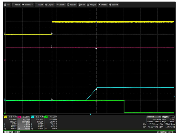
Figure 4: ivS1-3W0-3W0-1W0-70-A Turn-on Delay via Global Inhibit Vin = 180Vac Load: I_O = 66.88A I_{SB} = 1A Ch 1: Global Inhibit Ch 2: V_{SB} Ch 3: V_O Ch 4: Global DCOK
