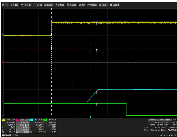
Figure 3: ivS1-3W0-3W0-1W0-70-A Turn-on Delay via Global Inhibit Vin = 90Vac Load: I_O = 31.25A I_{SB} = 1A Ch 1: Global Inhibit Ch 2: V_{SB} Ch 3: V_O Ch 4: Global DCOK
