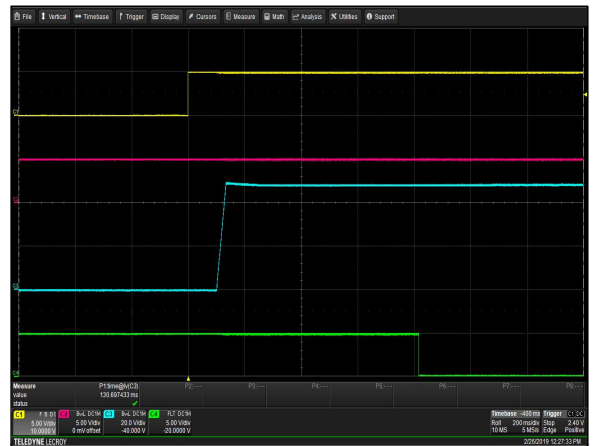
Figure 14: ivS6-3W0-3W0-1W0-70-A Turn-on Delay via Global Inhibit Vin = 264Vac Load: I_O = 66.5A I_{SB} = 1A Ch 1: Global Inhibit Ch 2: V_{SB} Ch 3: V_O Ch 4: Global DCOK
