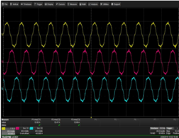
Figure 17: iVS6-3W0-3W0-1W0-70-A Input Current Waveform Vin = 170Vac Load: I_O = 66.5A Ch 1: I_{INL1} Ch 2: I_{INL2} Ch 3: I_{INL3}
