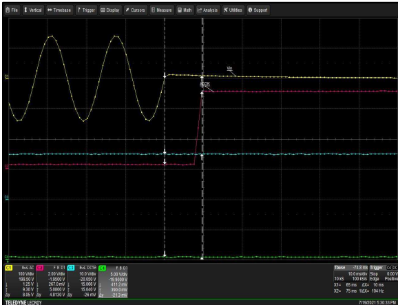
Figure 28: LCM600N ACOK Signal Turn-off Delay - V_{in} = 100V_{ac} Load: I_o = 2A (12V) , I_{SB} = 0A (5V) Ch 1: AC Mains Ch 2: ACOK Ch 3: V_o Ch 4: DCOK
