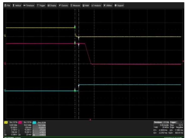
Figure 21: LCM600N Turn-off Characteristic via INH_EN Full Load: Io = 40A (15V), I SB = 2A (5V) Ch 1: INH_EN Ch 2: Vo Ch 3: POWER GOOD
