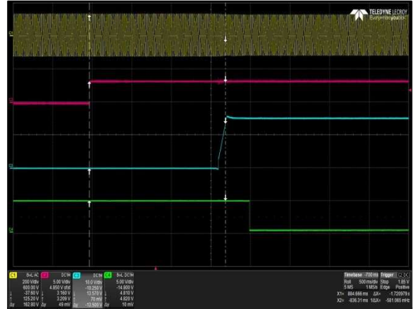
Figure 17: LCM600N Turn-on Delay via INH_EN - Vin = 90Vac Full Load: Io = 40A (15V), I SB = 2A (5V) Ch 1: AC Mains Ch 2: INH_EN Ch 3: Vo Ch 4: POWER GOOD
