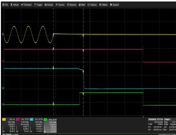
Figure 18: LCM600N Hold-up Time - Vin = 90Vac / 63Hz / 0° Full Load: Io = 40A (15V), I SB = 2A (5V) Ch 1: AC Mains Ch 2: V SB Ch 3: Vo Ch 4: POWER GOOD
