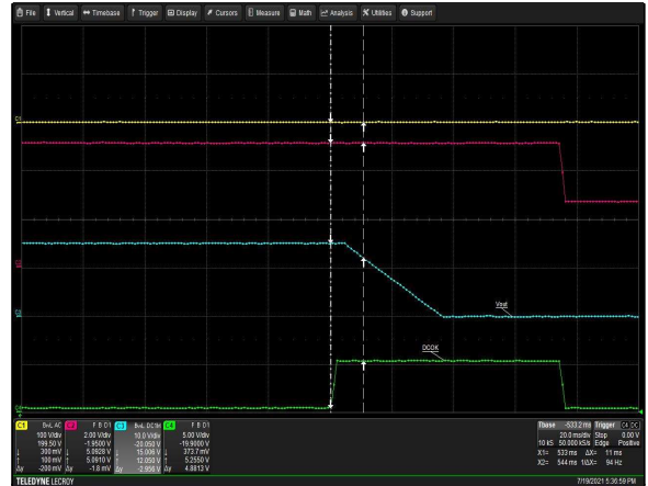
Figure 29: LCM600N DCOK Signal Turn-off Delay - V_{in} = 100V_{ac} Load: I_o = 2A (12V) , I_{SB} = 0A (5V) Ch 1: AC Mains Ch 2: ACOK Ch 3: V_o Ch 4: DCOK
