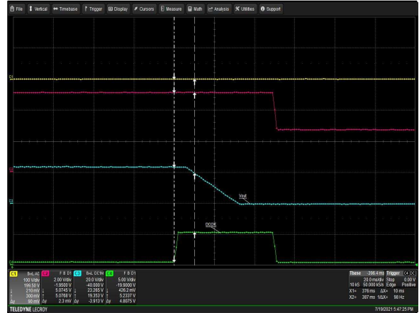
Figure 44: LCM600Q DCOK Signal Turn-off Delay - V_{in} = 100V_{ac} Load: I_o = 2A (12V), I_{SB} = 0A (5V) Ch 1: AC Mains Ch 2: ACOK Ch 3: V_o Ch 4: DCOK
