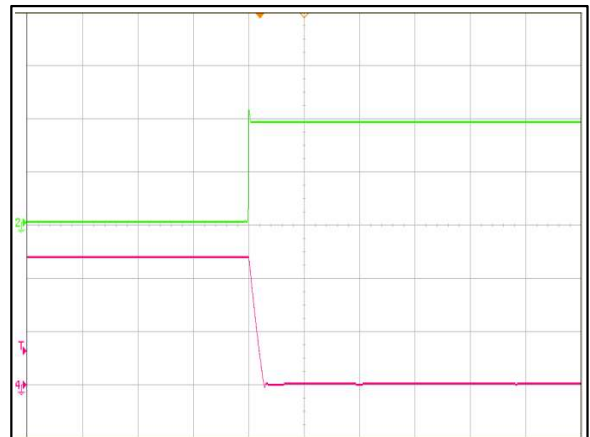
Figure 3: AVD75B-48S12 Output Voltage Shut Down By Remote Off V_{IN} = 48Vdc, I_O = I_{O,max}, 10mS/div Ch 2: Remote Off (2V/div) Ch 4: V_O (5V/div)
